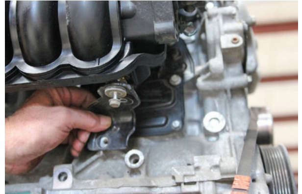
Figure 1: Removing the intake bracket.
