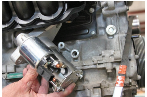
Figure 2: Rotating the starter nose to the 10 to 11 o'clock position.
