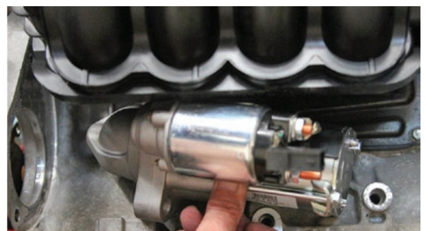
Figure 3: Raising the rear of the starter up and sliding the assembly to the bell housing.
